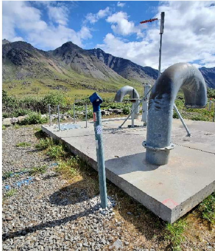
Fig. 7: Liquid hydrocarbon sensor featuring water level sensor
